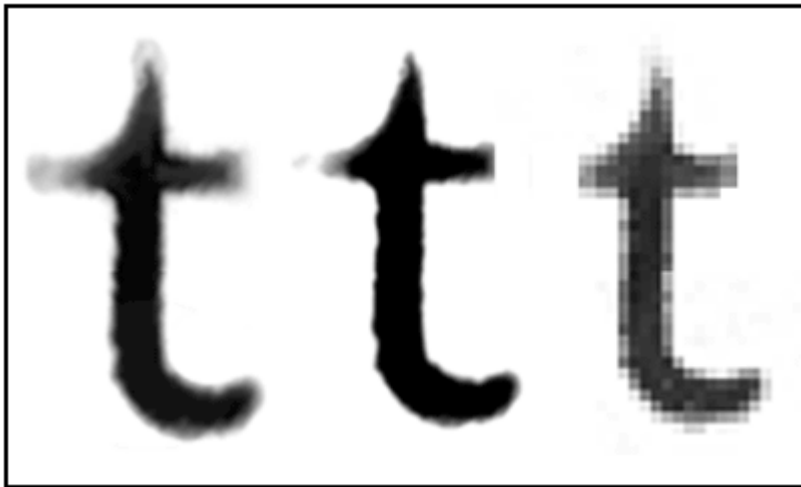
Figure 14. Letter “t” scanned in and artificially “worn” out; printed in high contrast; then rescanned in 72 pixel/inch resolution. Results are identical to comparable characters in the Bush memo.
