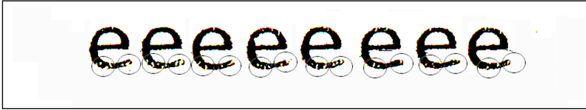
Figure 12. Damage can often become more apparent at high contrast. While the bottom of the characters show consistent damage, the left side of the bowl on the fourth “e” from the left shows damage caused by a defect in the ribbon or paper.
